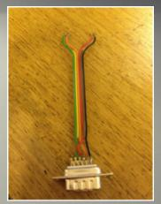
Use the controls lines present on many graphics card to interface I2C device
